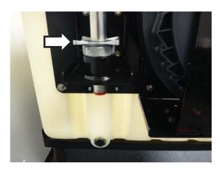
12. Connect the hose reel to the pump using the provided 1/2" hose, reducer bushing, and swivel 90°.
