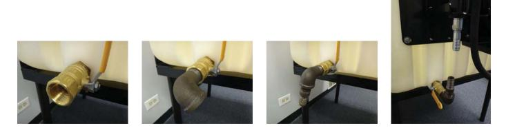
16. Measure, cut, and install a section of 1" hose between the two king nipples using two hose clamps. Use the pump's vertical adjustment to make hose installation easier.
