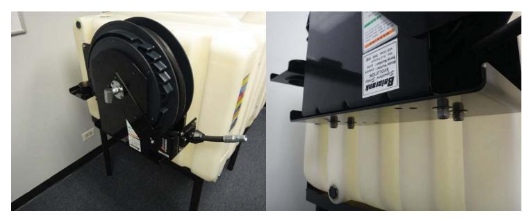
10. Fasten the pump's mounting nut onto the pump bracket.
