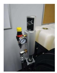
18. Install the fill nozzle onto the end of the dispenser.
