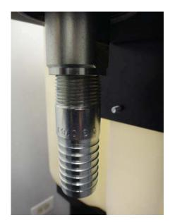
14. Remove the 1" NPT plug from the bottom left corner of the tank's left side.
