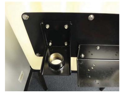
8. Reconfigure the hose reel using a hex key so that the hose will exit towards the tank's front.
