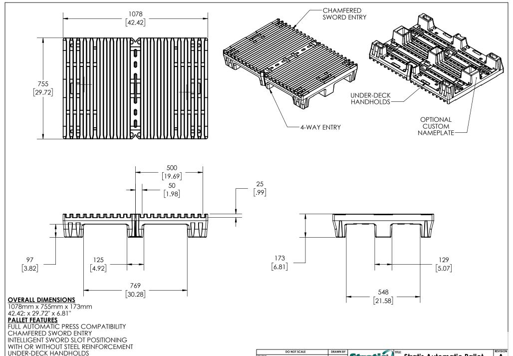
4-WAY ENTRY ALL DIMENSIONS ARE IN MM [INCHES], NOMINAL, & SUBJECT TO CHANGE WITHOUT NOTICE. ALL DIMENSIONS ON MOLDED PARTS ARE SUBJECT TO A  $\pm~2\%$  TOLERANCE.
