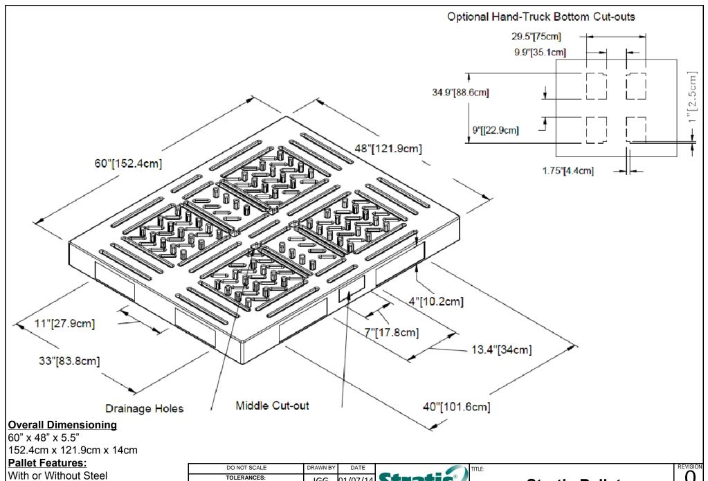
Reinforcement 4-Way Forklift Entry Bottom Cut-Outs for Hand-Truck Entry by request (add -CT to #)
