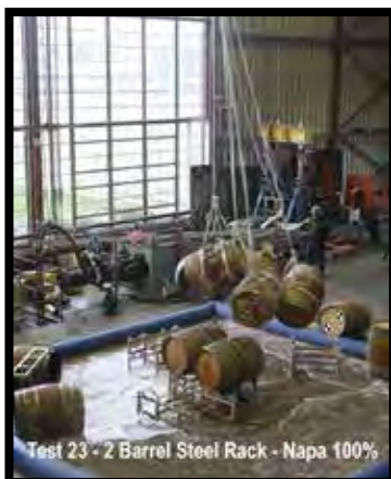
2 Barrel Steel Rack Fails 100% of the Napa quake simulation.
