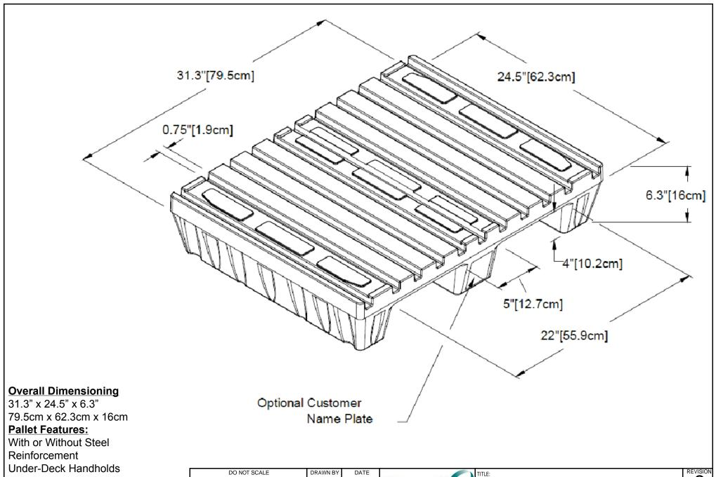
**Under-Deck Handholds** Deck-Lok Safety Stacking System Enhanced Flip-Flop Stacking
