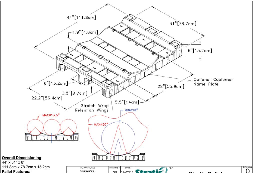
With Steel Reinforcement 2-Way Entry Under-Deck Handholds Stackable
