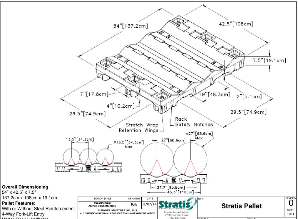
4-Way Fork-Lift Entry **Under-Deck Handholds** Stackable
